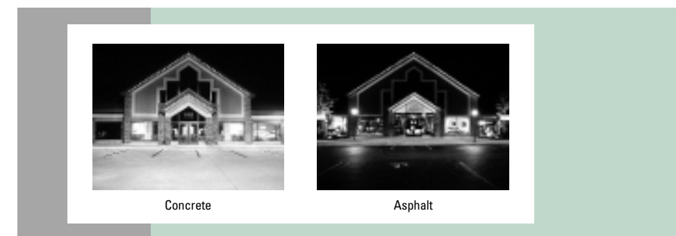
FIGURE 4 – LIGHTING ON CONCRETE AND ASPHALT SURFACES
